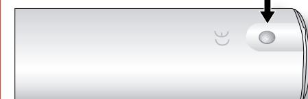
1. Open the battery compartment by pressing the button on the back of the handset.
